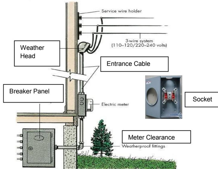
If a Field Service Representative observes a potential **Unsafe Condition** at your location: **loose, rusted, or worn meter socket, or worn entrance cable** that is in need of replacement or repair. This is an unsafe condition for you as a homeowner as well as the public. In addition, **Meter Clearance from bushes, vines, fences, or storage items** must be rectified before service is energized.
